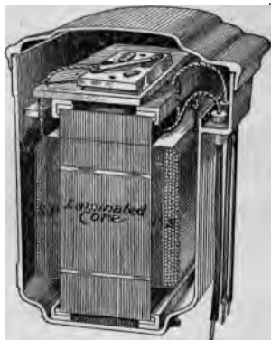
FIG. 424. — Commercial Transformer. P, P , primary coil; S, S , secondary coil.
