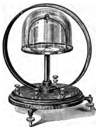
FIG. 352. — Tangent Galvanometer, a Fixed Coil Instrument.
