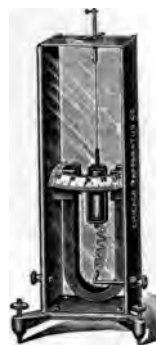
FIG. 353. — D'Arsonval Galvanometer, a Movable Coil Instrument.
