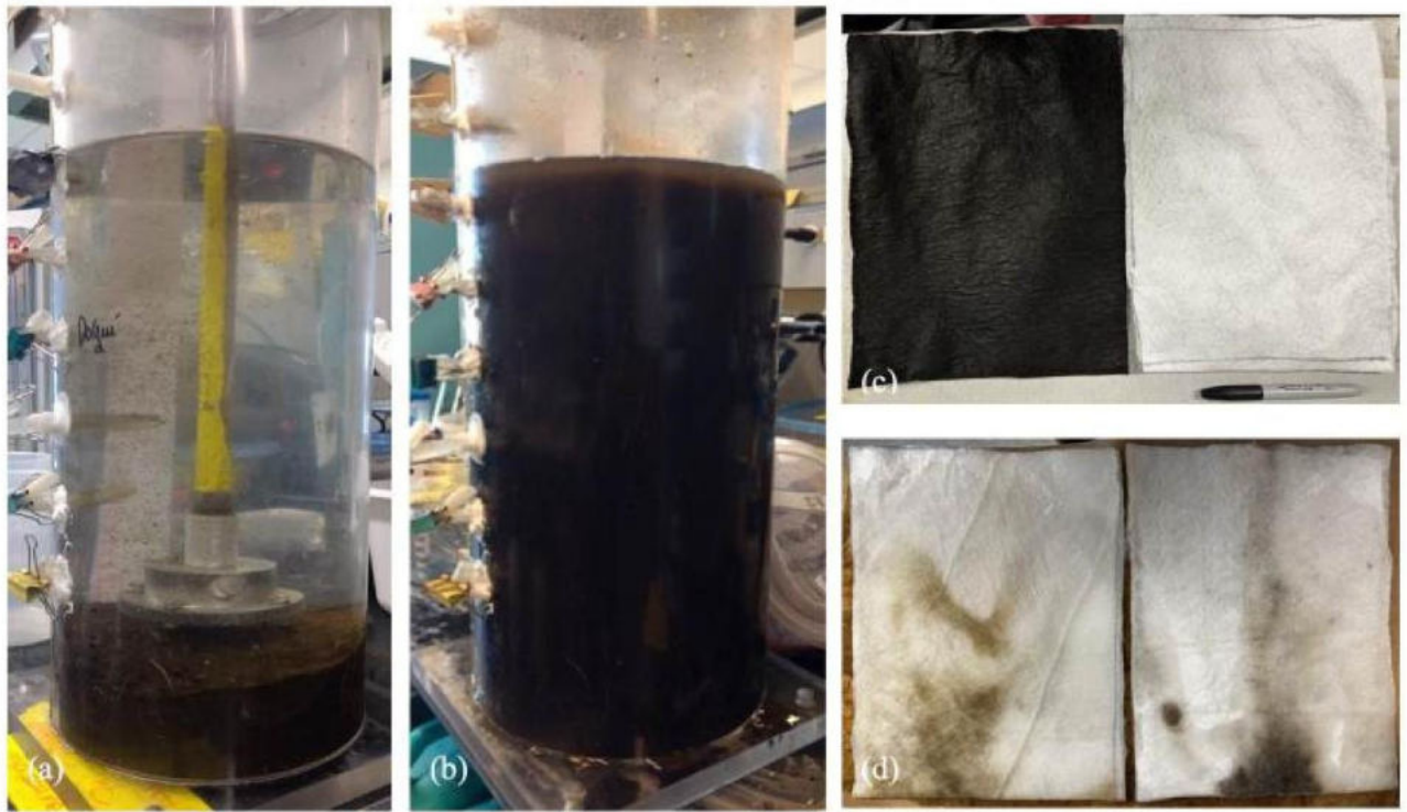
Fig 2. Sediment resuspension setup including: (a) sediment before resuspension, and (b) 0.5 min after resuspension and the (c) geotextile bag combination before the filtration process and (d) after the filtration process.
