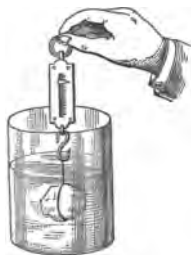
FIG. 73. — The water supports a part of the weight of the stone.
