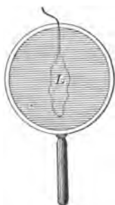
FIG. 13. — An equal surface tension within and without the loop L .
