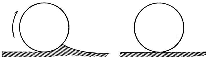
FIG. 115. — As a body rolls on a plane surface, both are deformed slightly.
