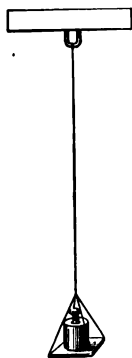
FIG. 11. — The tensile strength of the wire is shown by the load it will carry.
