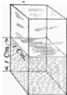
FIG. 41 b. — Water 1 cm. deep exerts a pressure of 1 gm. per sq. cm.
