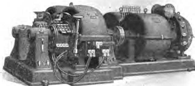
FIG. 234. — Compound turbine engine coupled directly to a dynamo.
