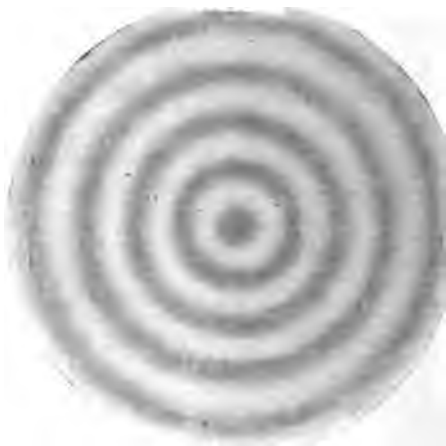
FIG. 245. — A section through a wave train, showing at a given instant the alternate condensations and rarefactions in the air which travel outward from the center with the speed of sound.
