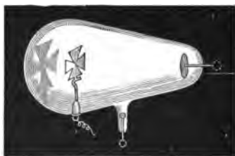
FIG. 426.—Cathode rays producing a shadow.
