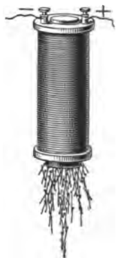
FIG. 367.—An electromagnet. Straight form with soft iron core.
