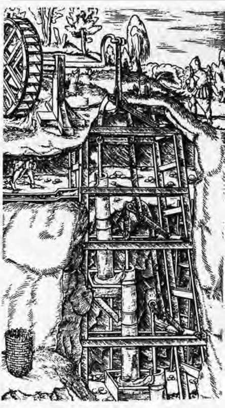
▼ Figure 3.5 The book De re metallica , by AGRICOLA (GEORG BAUER, 1494–1555), was an epoch-making event in mining and metallurgy. Of particular interest for us are the methods of measurement described and, above all, the construction of multistage pumps. The Scholastic problem of horror vacui has here become a technical problem.
